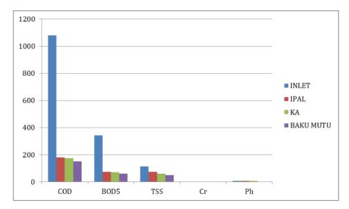
The histogram image of the test results between the textile industry wastewater from the inlet, Outlet PT. SSI Sukoharjo, Quality Standards for liquid waste and with using activated carbon filtering.
